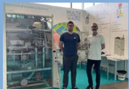
Secma Cabon of France exhibited its Multi-Ways automated feeding system that evenly distributes feed across the water surface. It's computer controlled allowing for frequent daily feeding schedules in multiple ponds. The manufacturer says its enhanced the FCR while improving water quality of both the ponds and the discharge water. It helps to maintain pellet integrity with no fines
