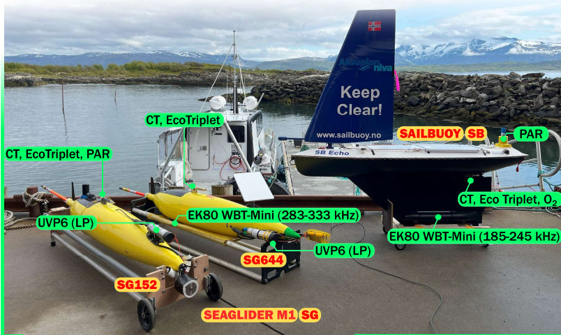
The fleet of autonomous vehicles deployed during 2025 spring campaign (c) Pierre Priou
